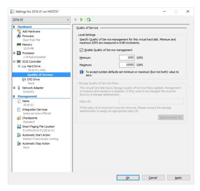
Alternatively, the minimum and maximum IOPS for a disk can be set by using the Set-VMHardDiskDrive cmdlet. For example, to set the maximum IOPS of the SCSI disk associated with VM1 to 5000 and the minimum IOPS to 500, run the following command:
